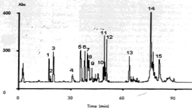
Figure 4. Tryptic digestion and RP-HPLC of IFN- $\alpha_{2b}$ . For details, see Materials and Methods. Mass/charge ratio ( $m/z$ ) of different peaks are: 1, 613.0; 2, 618.0; 3, 740.9; 4, 902.8; 5, 750.1; 6, 1450.0; 7, 2225.8; 8, 1955.3; 9, 1481.6; 10, 1076.6; 11, 910.4, 1337.4, 2245.5, 1337.4, 2245.5; 12, 910.3, 1209.2, 2117.1; 13, 1313.3, 3303.6, 4617.1; 14, 1313.4, 4737.0, 6049.4; 15, 2459.7 [21].
