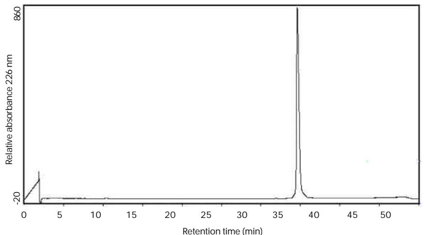
Figure 3. RP-HPLC analysis of recombinant IFN- $\alpha_{2b}$  preparations was performed using a Bakerbond wide pore octyl (C8) column equilibrated with solution A (0.1% TFA). Elution was carried out with solution B (0.1% TFA in acetonitrile) from 0% to 6% (v:v) in 50 min.
