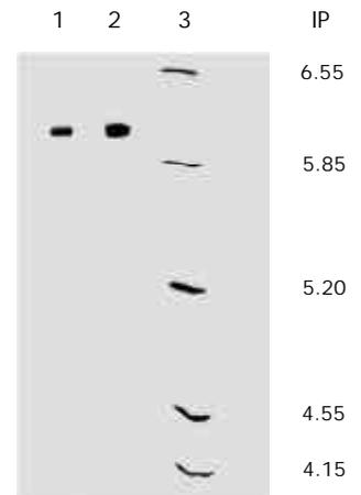
Figure 2. Isoelectric focusing of IFN- $\alpha_{2b}$  (CIGB) as described in Materials and Methods. Lanes 1 and 2, 5 and 10  $\mu\text{g}$  of IFN- $\alpha_{2b}$  (CIGB), respectively; lane 3, isoelectric point marker (IP) for the valves, 6.55, 5.85, 5.20, 4.55, 4.15 (the most alkaline is near the application point).
